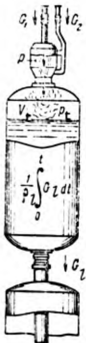
Figure 15. Diagram of the tank pressurizing system.
