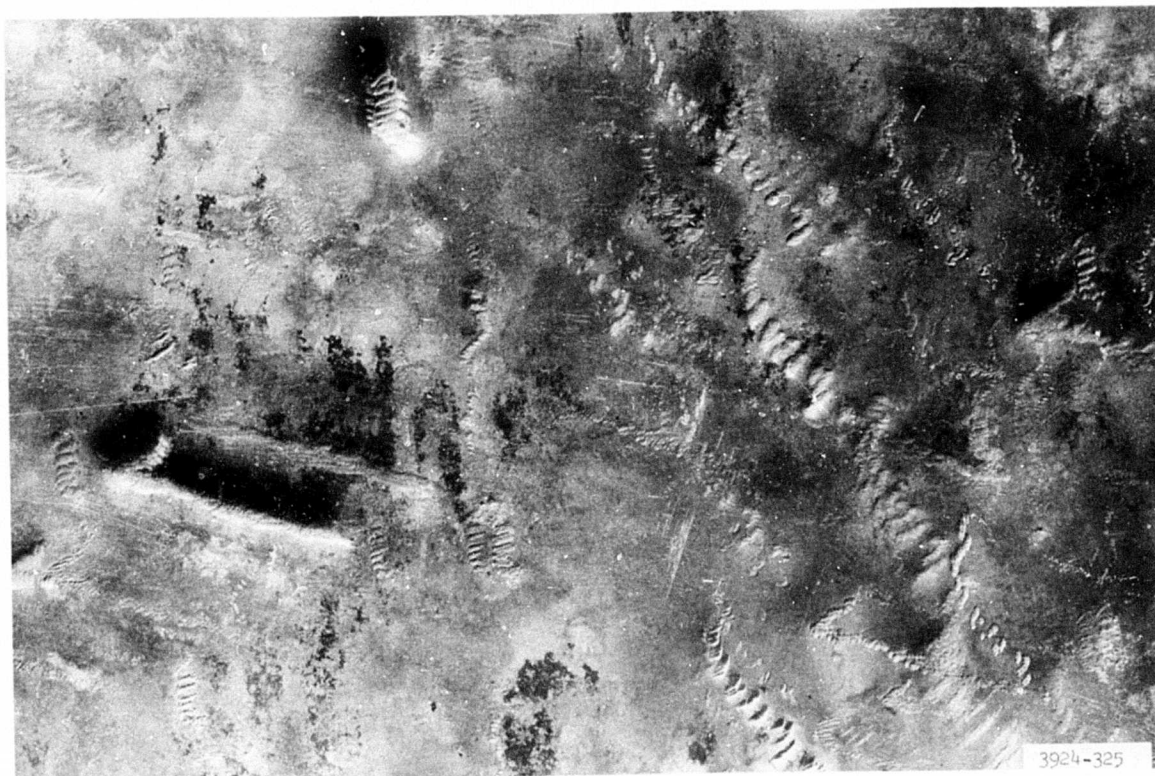
Photograph 67. Indentations on underside of mat that had been placed on clay gravel
