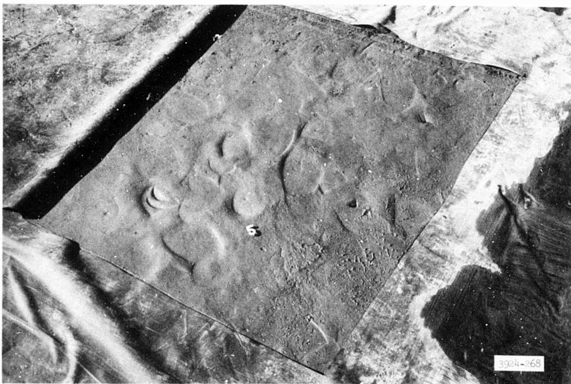
Photograph 64. Lean clay directly under holes shown in photograph 63
