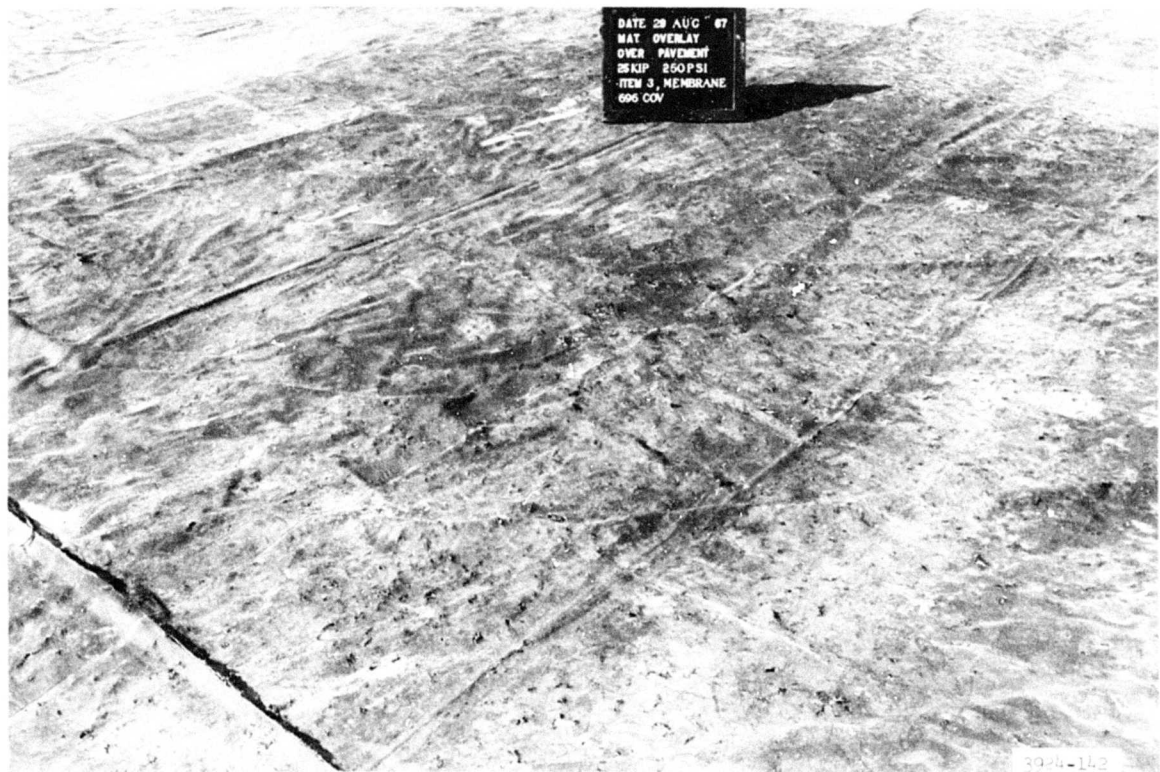
Photograph 44. Numerous holes worn in T16 membrane on item 3 during 366 coverages (696 total coverages on section)
