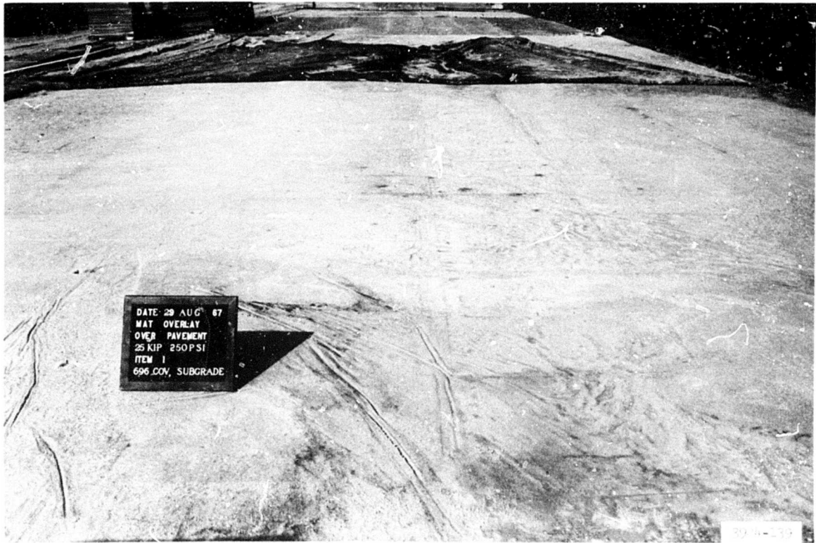
Photograph 43. Condition of sand overlay in item 1 after 696 coverages
