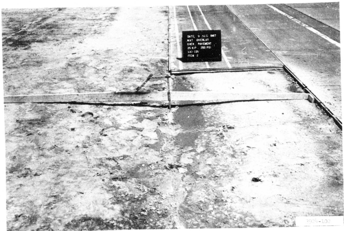
Photograph 30. Condition of sand overlay after 330 coverages
