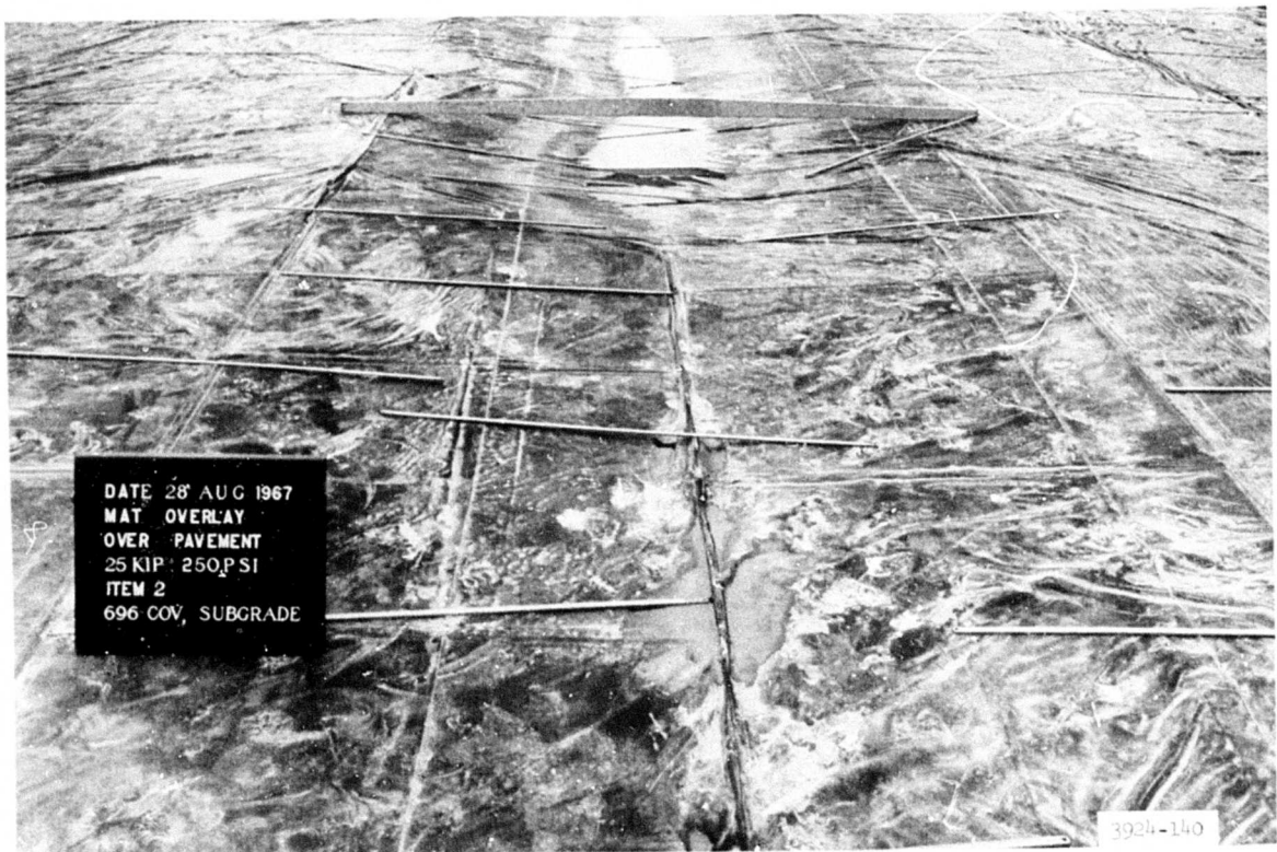
Photograph 42. T16 membrane in item 2 after mat was removed after 696 coverages (rods are XM19 connector bars)
