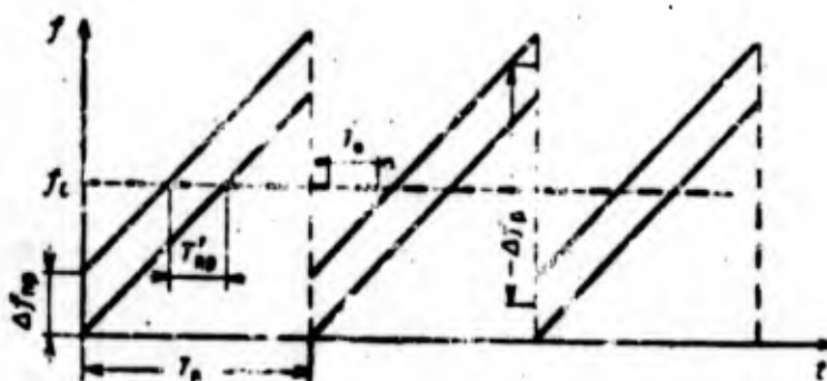
Fig. 10.5. Frequency-time diagram, explaining a slow scanning of frequency.
