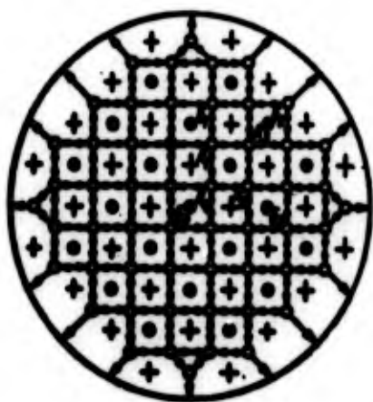
Fig. 3.33. Formation of bundles at head with checkerboard placement of injectors: \bullet - oxidizer injectors; + - fuel injectors; \circ - points of formation of bundles.
