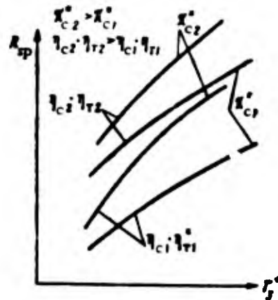
Fig. 1.14. Character of variation of specific thrust R_{sp} versus gas temperature T_3^* for various values of the product \eta_c - \eta_T .
