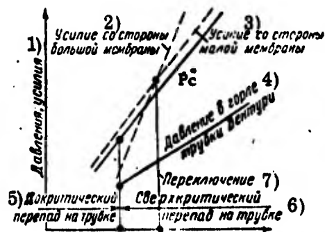
Fig. 2.48. Plots of air pressure variation at inlet and throat of Venturi tube.
