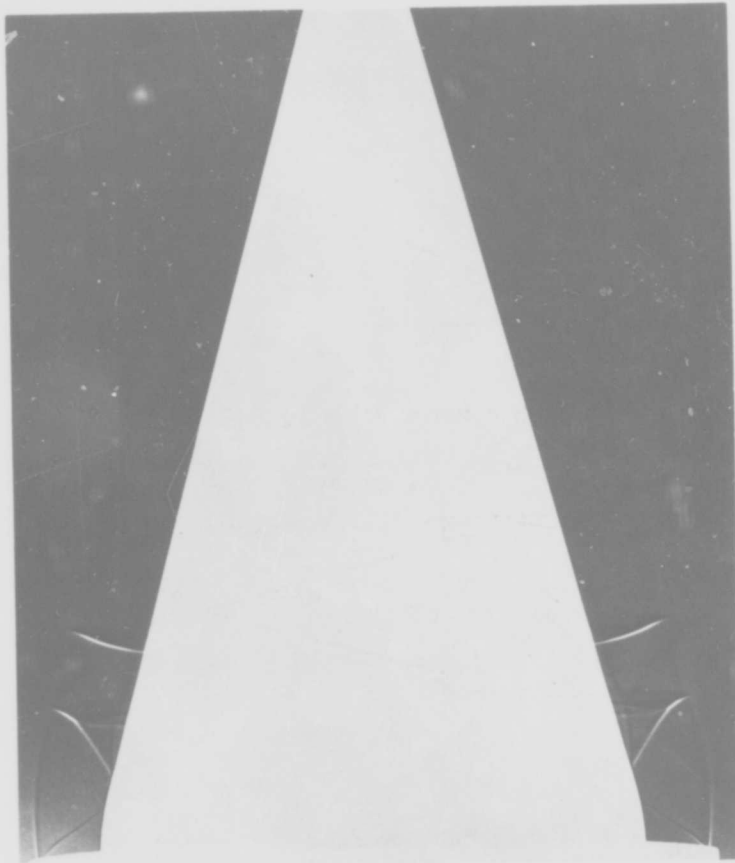
FIG 12 SHOCK WAVES ON PLUG NOZZLE
