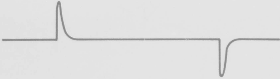
Fig.6. Calculated waveform from a uniform explosive line charge
