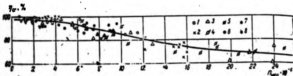
Fig. 50. Combustion completeness \eta_{sc} versus vaporization parameter \Pi_{iscn} ( \alpha_1 = 1.2-1.5 , t_0 = 200-290^\circ\text{C} , t_{k,c} = 700-750^\circ\text{C} , fuel is solar oil, distillate oil, M-20 fuel oil): 1) ГТ-100-750, D_{n,r} = 640 mm; 2) ГТ-100-750, D_{n,r} = 400 mm; 3) block of combustion chambers ГТ-100-750, D_{n,r} = 270 mm; 4) ГТУ-4-750 КТЗ, D_{n,r} = 270 mm; 5) ГТ-1.5-700 НЗЛ, D_{n,r} = 305 mm; 6, 7, 8) experimental chambers, D_{p,t} = 400, 360, 540 mm, respectively.
