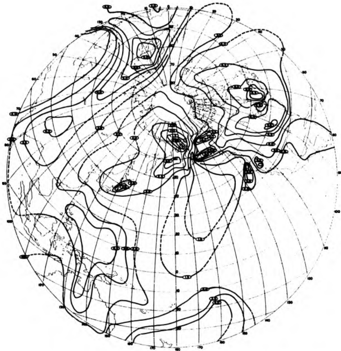
Figure 24. Contours of negative JB travel-time residuals for LONG SHOT - equidistant azimuthal oblique polar projection from Amchitka Island.
