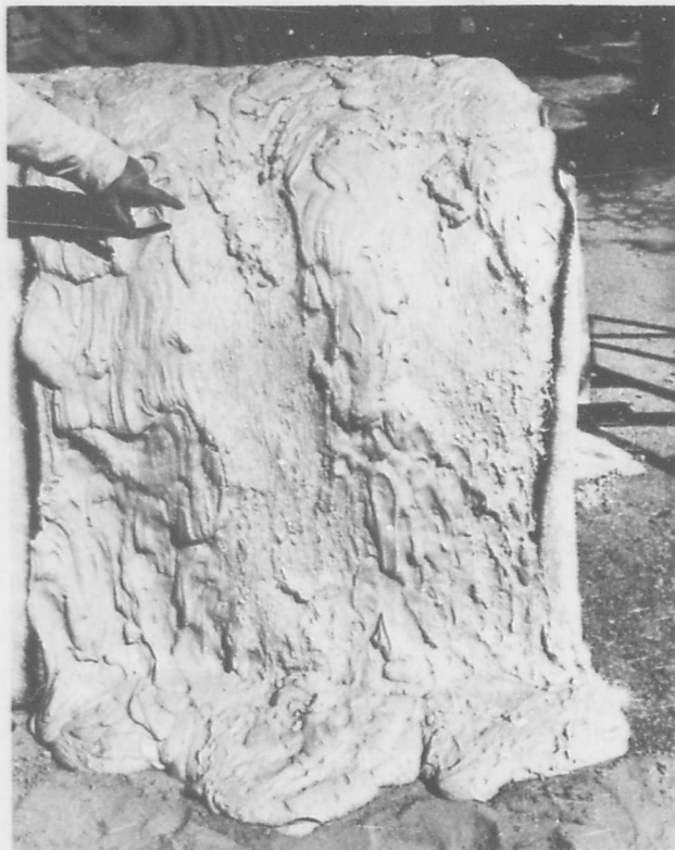
Figure 5. Flow of sulfur foam on near vertical wall.
