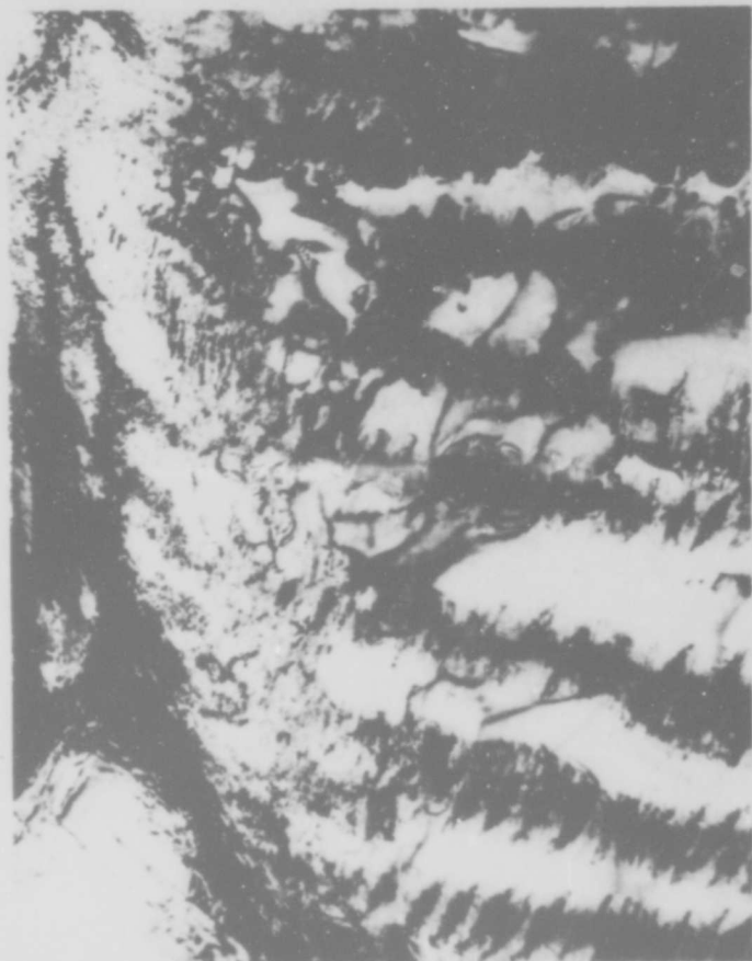
Figure 3. Electron micrograph showing the complex (high dislocation density) structure of Mill Annealed (1300°F/Air Cooled) Ti 6Al-6V-2Sn. No exposure.
