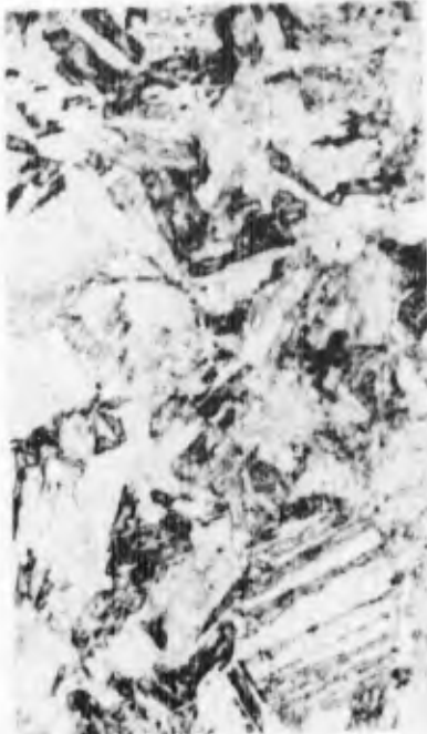
SOLUTIONED AT 1700°F AGED 3 HRS AT 950°F MAGNIFICATION 500X FRY'S ETCH
