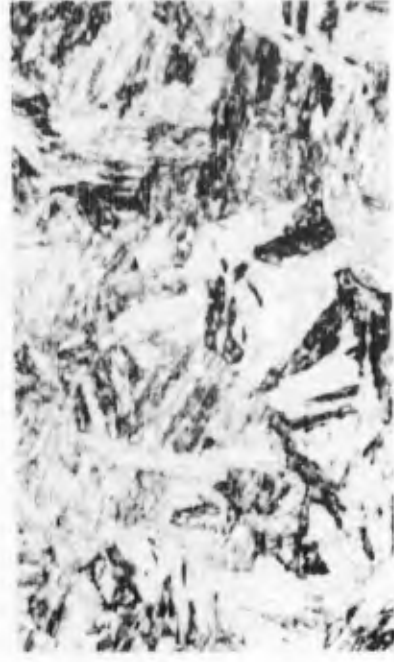
SOLUTIONED AT 1800°F AGED 3 HRS AT 950°F MAGNIFICATION 500X FRY'S ETCH
