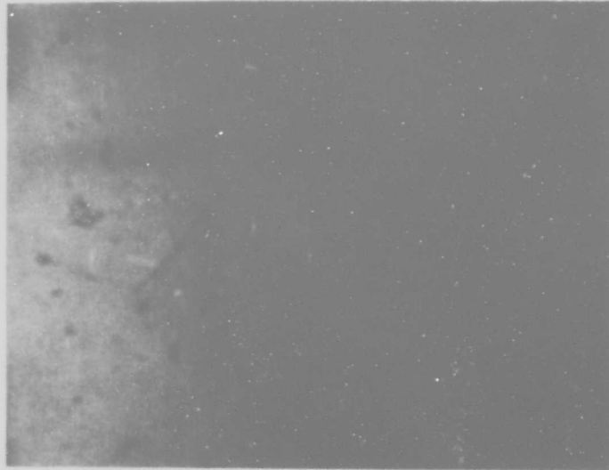
Figure 13. Ta-N (65-35 At.%), Melting Point Sample Quenched from 2955°C. X1000
