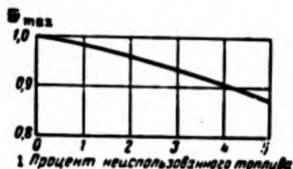
Fig. 1.10. Influence of underutilization of fuel supply on maximum rocket speed. 1) Percent unused fuel.
