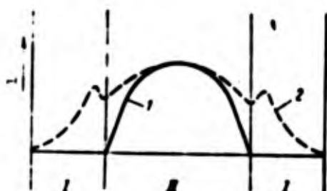
Fig. 11.4. Change of neutron flux in a reactor with a reflector and without it: I - reflector; II - cores; 1 - without reflector; 2 - with reflector.
