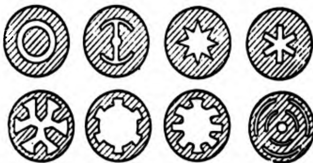
Fig. 5.14. Certain grain shapes with internal burning.
