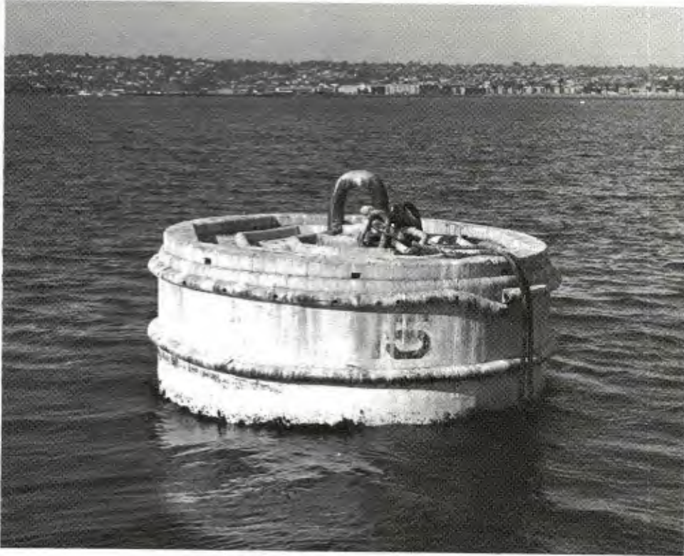
Figure 2. Hand lay-up buoy in San Diego Bay after 4 years of service. Note guano staining on side and slight displacement of upper lateral fender.
