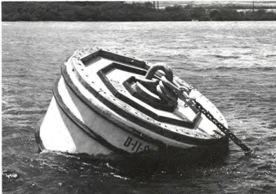
Figure 7. Plastic buoy after 1 year of service at Pearl Harbor.
