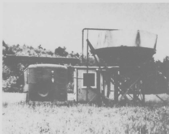
Fig. 2. Photograph of the radar. The radar site was surrounded by wooded hills which suppressed disturbing side-lobe radiation. Further suppression of side-lobe ground-echoes was obtained by mounting a metallic collar along the rim of the antenna. The circular parabolic antenna had a 4-m diameter and was fixed with the beam axis in the vertical direction.
