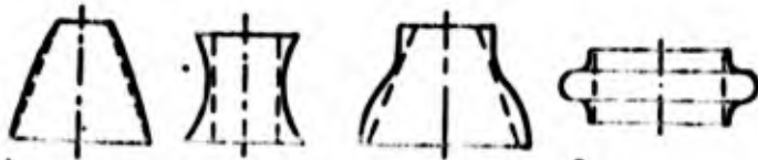
Fig. 2.13. Standard parts obtained by stretching by a releasing punch.
