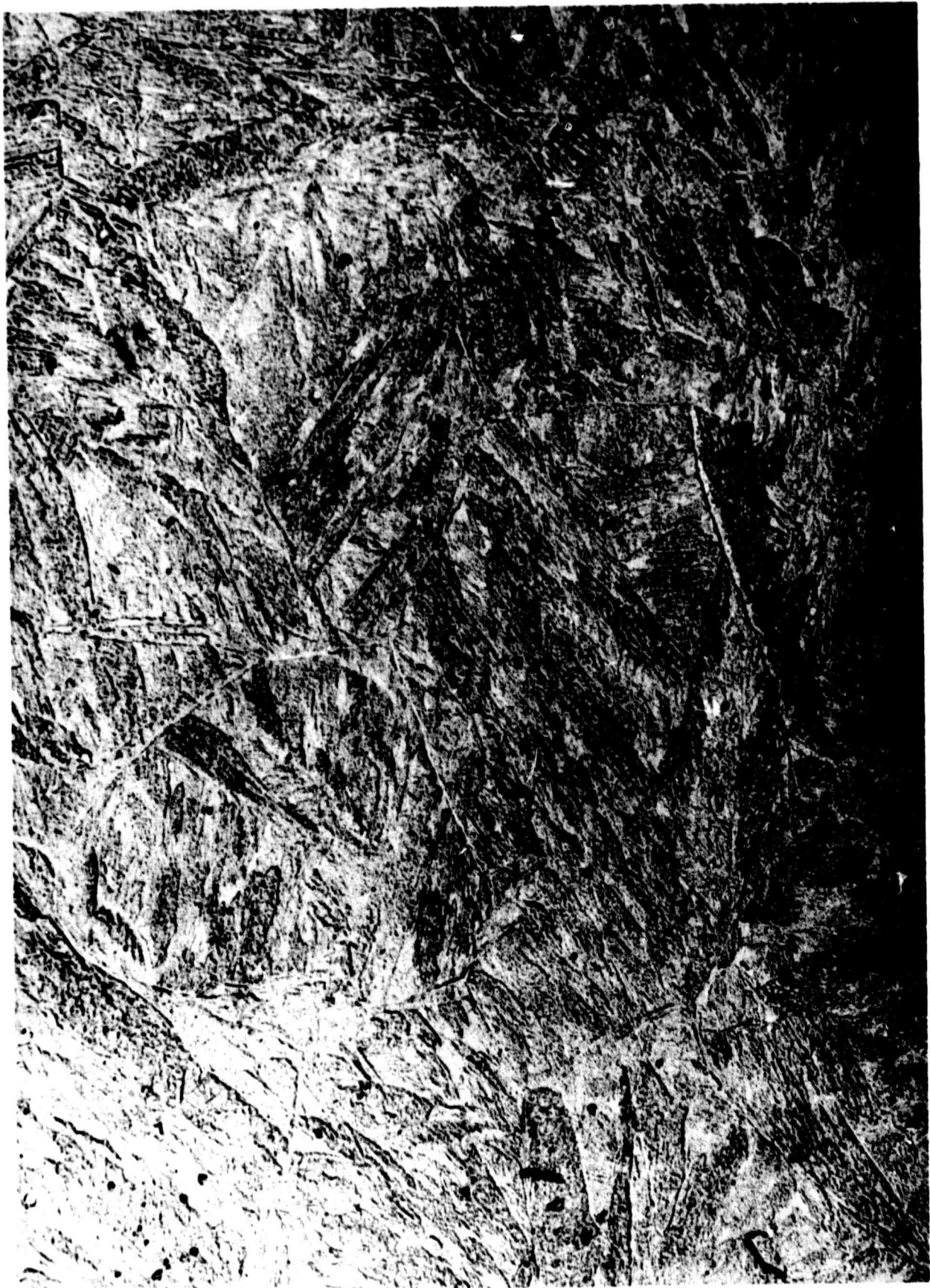
Figure 8 4340M: tempered 1 hr at 1275°F, cold reduced 50%, and austenitized 1 hr at 1550°F. Few undissolved carbides remain. Extraction replica (X12,000).
