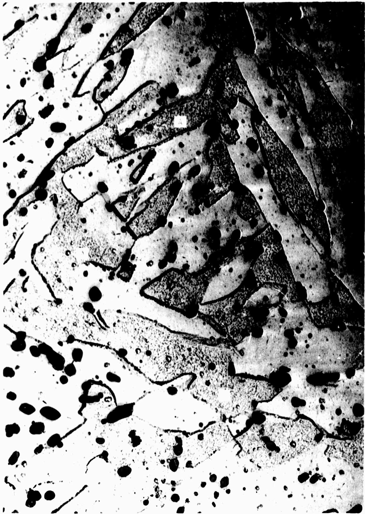
Figure 2 4340M: undeformed tempered martensite austenitized 1 hr at 1325°F and water quenched. Acicular, newly formed austenite is marked A in background of recrystallized ferrite. Undissolved carbides are pinning the phase boundaries. Extraction replica (X30,000).
