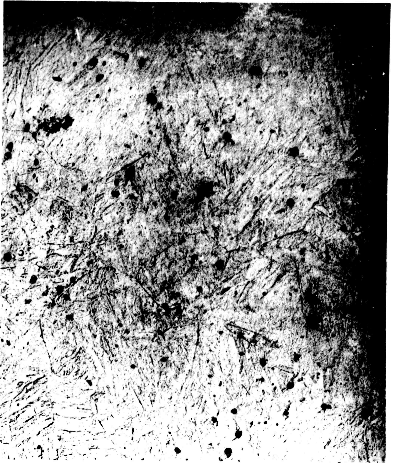
Figure 7 4340M: tempered 1 hr at 1275°F, cold reduced 50%, and austenitized 1 hr at 1525°F. Undissolved carbides remain. Extraction replica (X12,000).
