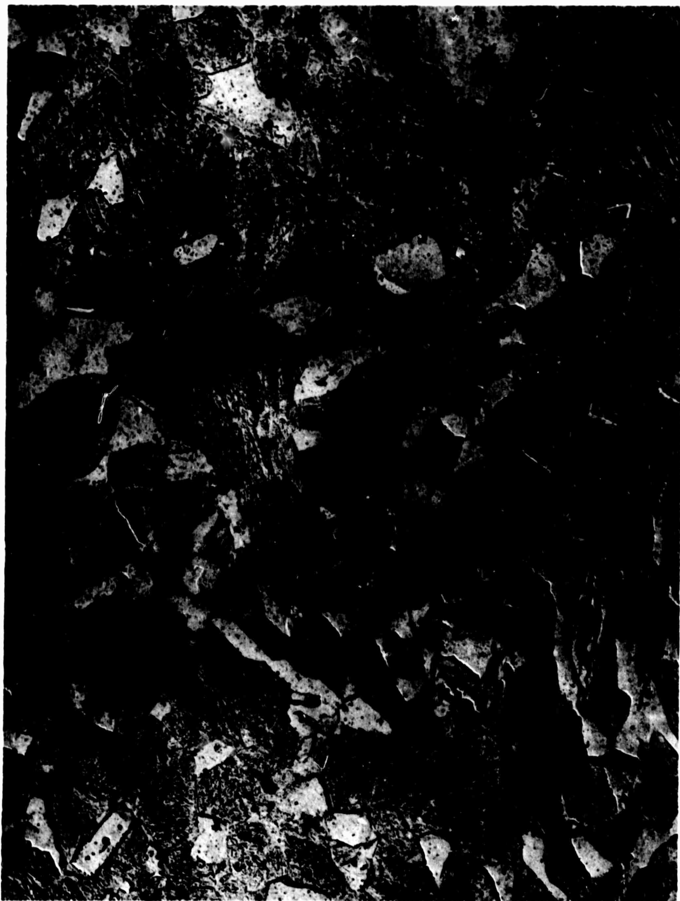
Figure 6 4340M: tempered 1 hr at 1275°F, cold reduced 50%, austenitized 1 hr at 1480°F, and water quenched. Blocky ferrite lies at the boundaries of fine, equiaxed austenite grains. Extraction replica (X12,000).
