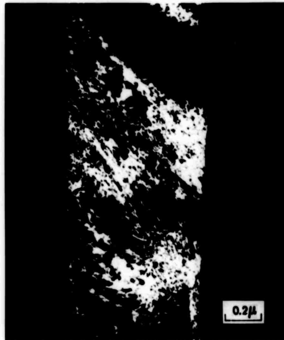
(a) At 2% uniform elongation. Zone normal \sim \langle 111 \rangle_{\beta} g = (0\bar{1}1)_{\beta} . Dark field.
