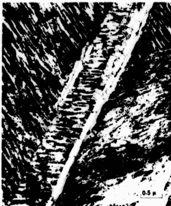
(c) \alpha -phase precipitation on first-order and second-order twin interface. Specimen was deformed 5% then aged 250 hr at 1150°F. Zone normal = \langle 311 \rangle_{\beta} . Bright field.
