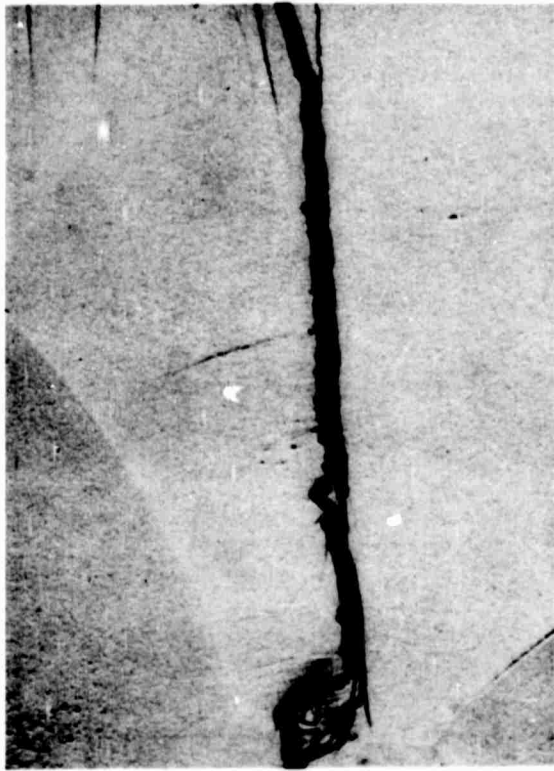
(a) Crack mode 1—cleavage type (x500).
