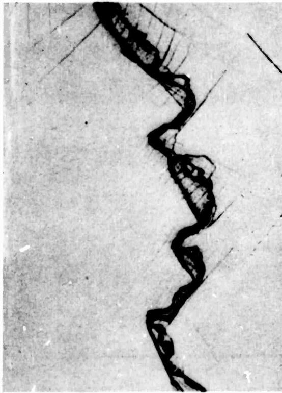
(b) Crack mode 2—discontinuous type (x500).
