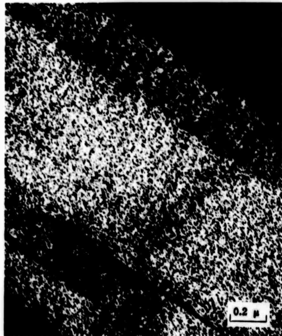
(b) \omega -phase particles within a deformation twin in a specimen deformed 2% then aged 30 min at 700°F. Zone normal = \langle 110 \rangle_{\beta} g = (0001)_{\omega} . Dark field.
