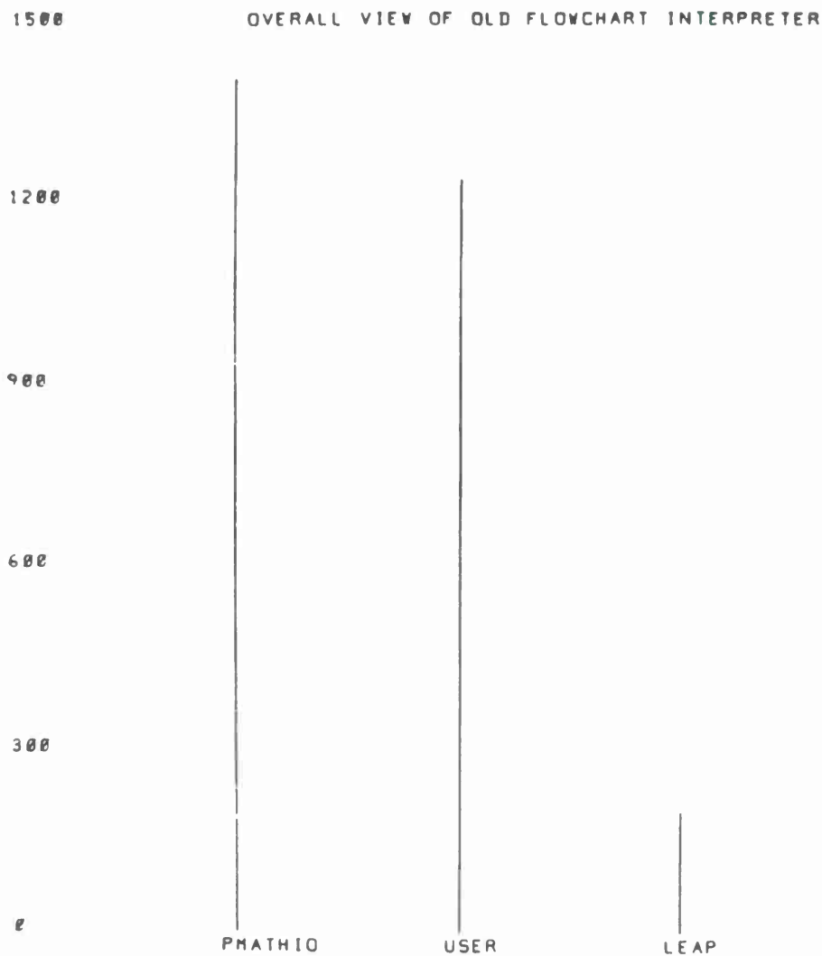
Fig. 2. This graph, photographed directly from the Tektronix 611 storage tube, shows the total number of instructions executed in each of three blocks of core during the interpretation of the flowchart in Fig. 1. Each unit on the vertical axis represents 2500 instructions executed.
