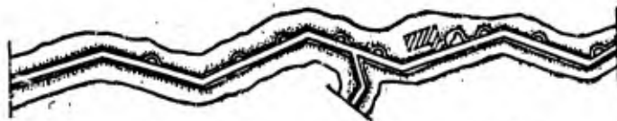
Digging connecting trenches to adjacent units and to the rear
