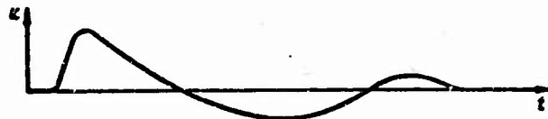
Fig. 2. Typical form of mass-velocity trace of compression wave in rock.
