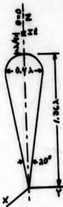
Figure 7. Radiation gain patterns for electric dipoles \lambda/4 from the sphere end of a conducting cone-sphere.
