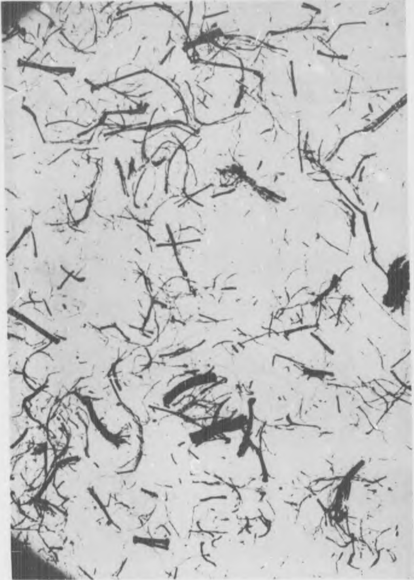
PLATE 6 GRADE 4 CHRYSOTILE (N 562 5R) Magnification x 12
