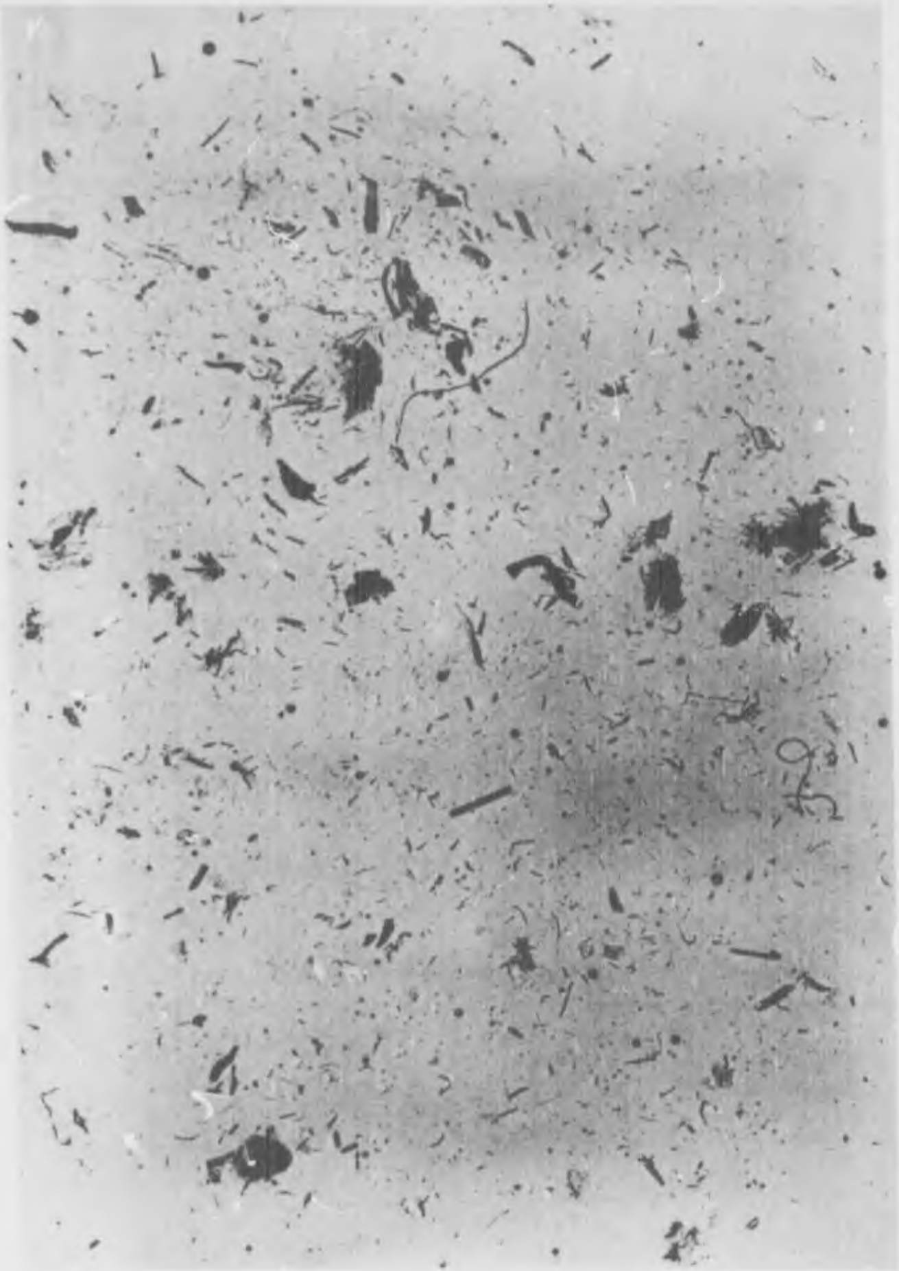
PLATE 12 RECOVERED CHRYSOTILE (N 562 5R) 28% GRADE (1-4) IN POLYPROPYLENE. Magnification x 20
