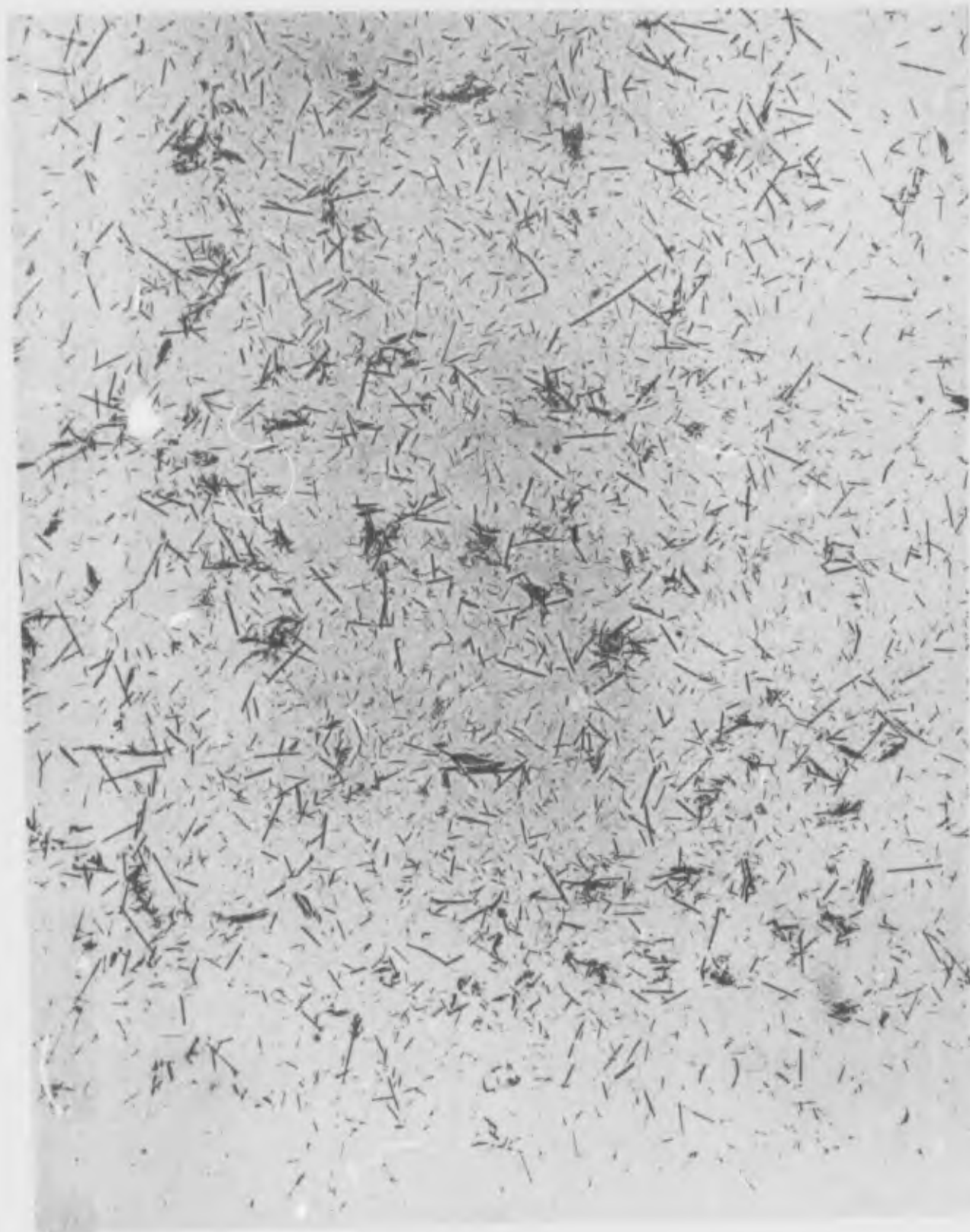
PLATE 9 RECOVERED CHRYSOTILE (C & GOB), 16% GRADE 1 IN POLYPROPYLENE. Magnification x 20
