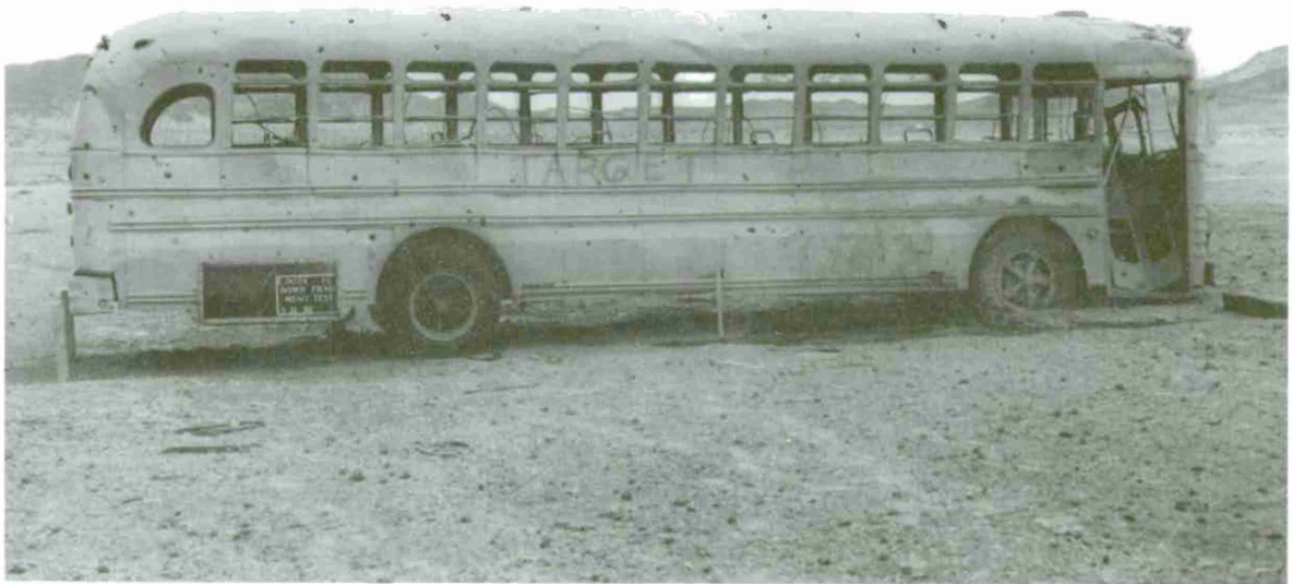
Figure 17. Damaged Bus Following the Test at China Lake.
