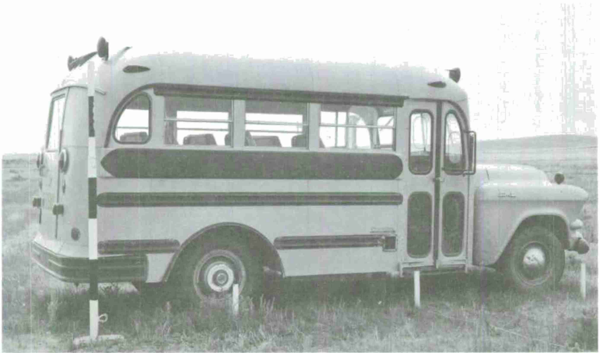
Figure 9. The Small Bus Set in Place at 3000 Feet From the 500 Ton Charge.
