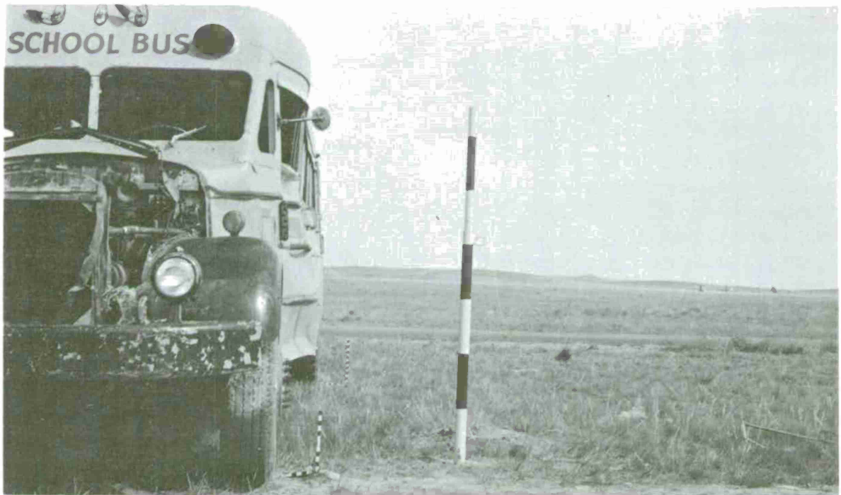
Figure 23. Damage to the Large Bus Following the Dial Pack Test - Front View.
