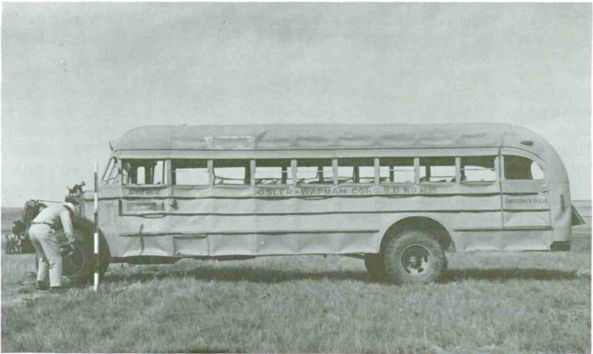
Figure 22. Damage to the Large Bus Following the Dial Pack Test - Side View.
