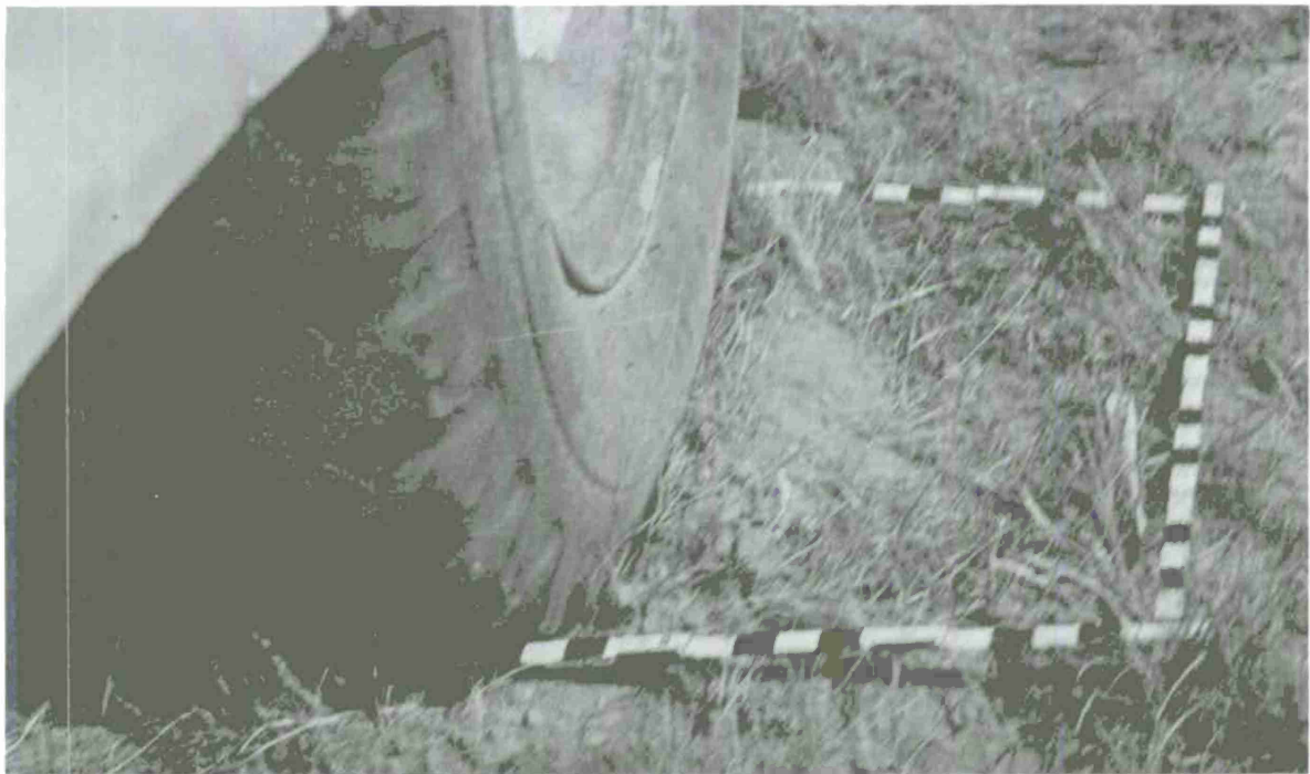
Figure 21. Up-Stream Tire and Soil Following Bus Rotation.
