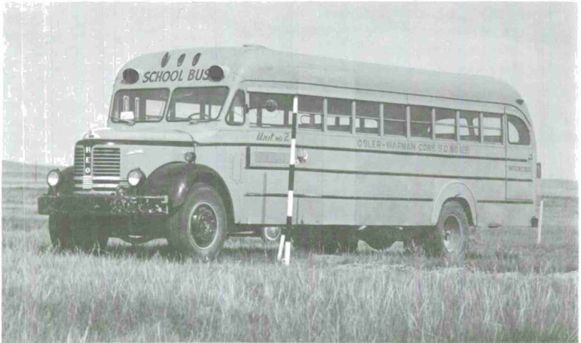
Figure 8. The Large Bus Set in Place at 1200 Feet From the 500 Ton Charge.
