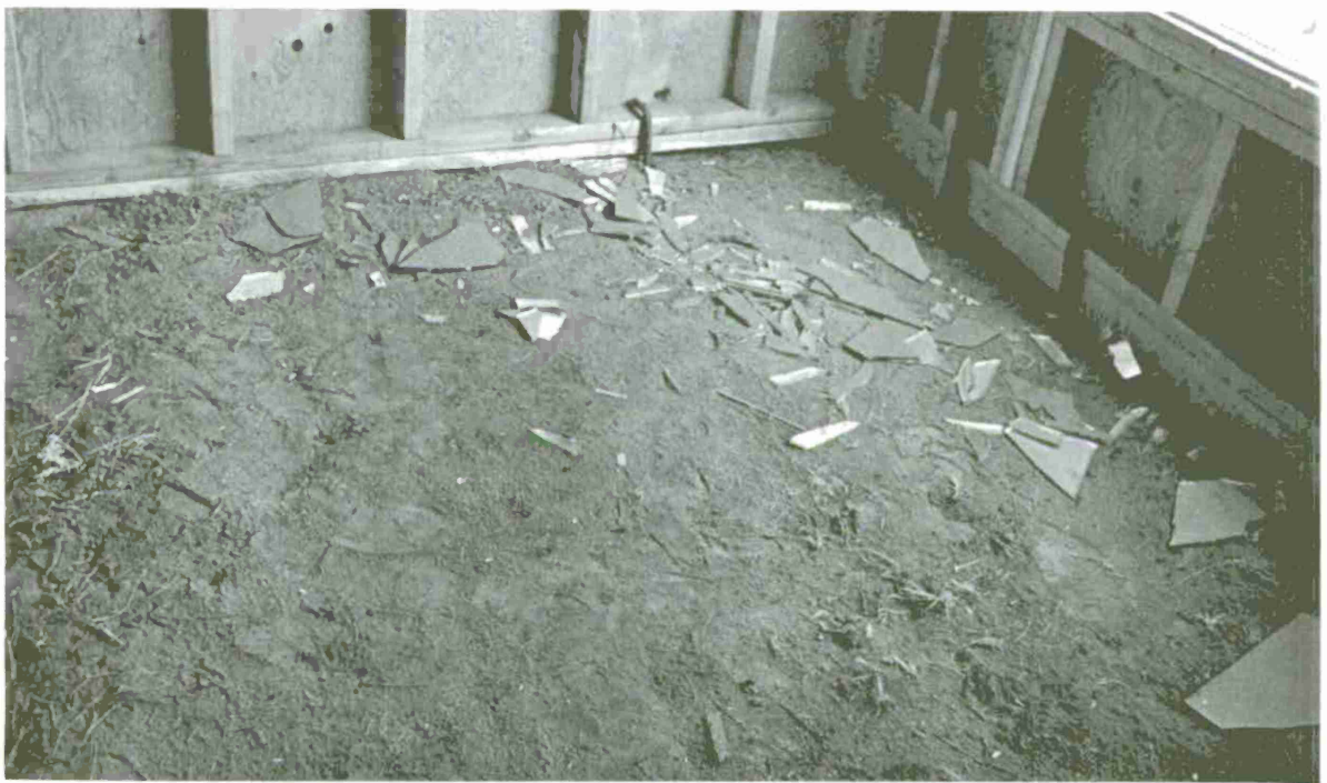
Figure 15. Glass Fragment Distribution Inside the Structure.
