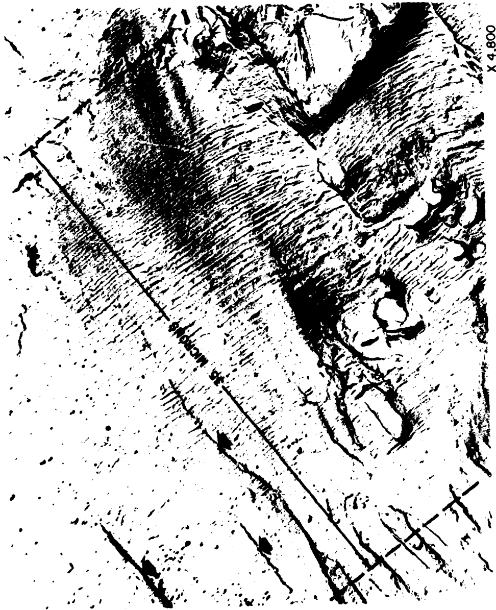
FIG. 2 ELECTRON MICROGRAPH OF THE FRACTURE SURFACE TOPOGRAPHY OF ONE MACROSCOPIC BAND
