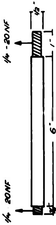
TESTING SHAFT (PART #13)
