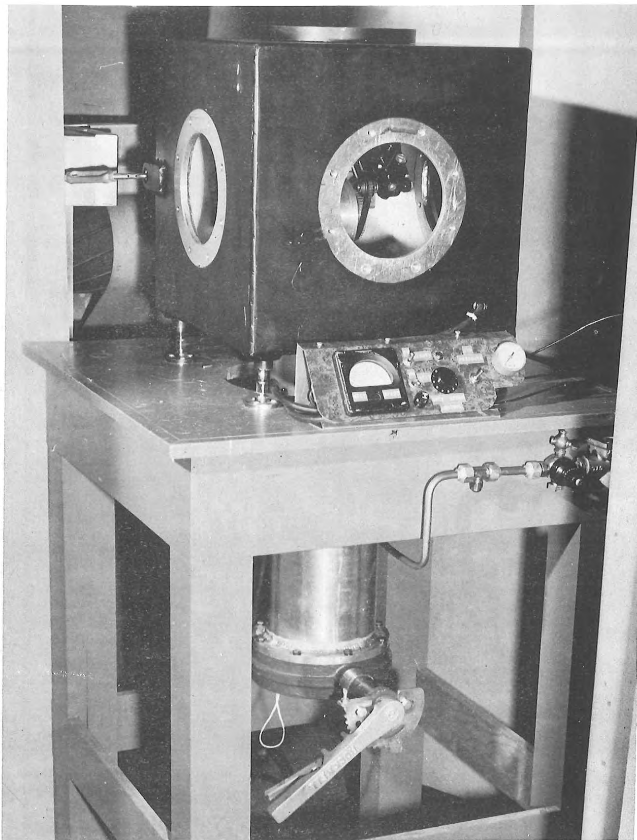
FIG. 10: View of exit end box with control panel and cooling receiver attached below.
