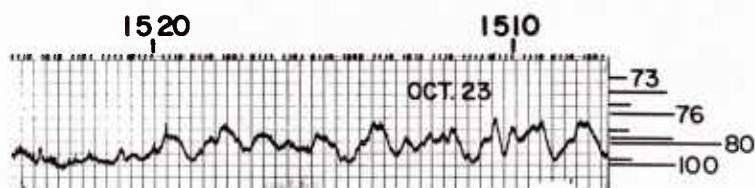
(c) SHOWS SLOW RELATIVELY SHALLOW SCINTILLATIONS CHARACTERISTIC OF THE PERIOD AROUND LOCAL NOON; FADES ARE OF THE ORDER OF 4-9 dB WITH THE PERIOD OF FADING 20-40 SECONDS.
