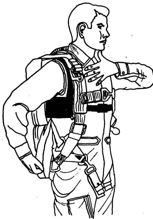
Figure 7. Parachute Harness and LPU Underarm Life Preserver Properly Integrated and Fitted
