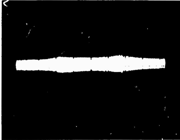
Figure 23a. Barkhausen noise induced in a specimen encircling 200 turn search coil during a traversal of the hysteresis loop. The specimen is a 1/4-in. -diameter rod of polycrystalline, 3% Si-Fe. The vertical sensitivity is 50 \mu\text{v}/\text{cm} and the horizontal time scale is about 5 sec/cm.
