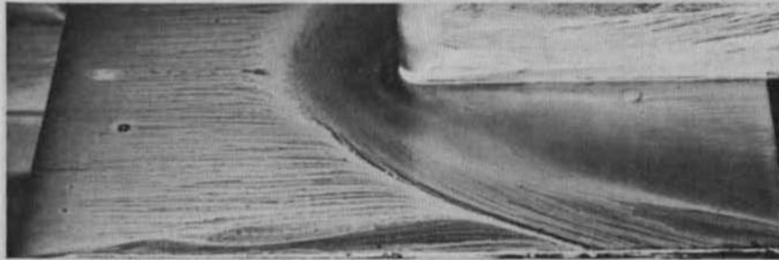
Configuration 0.750, M_\infty = 4.00 , Re_{x_F} = 2.8 \times 10^6 , Without Boundary Layer Trips
