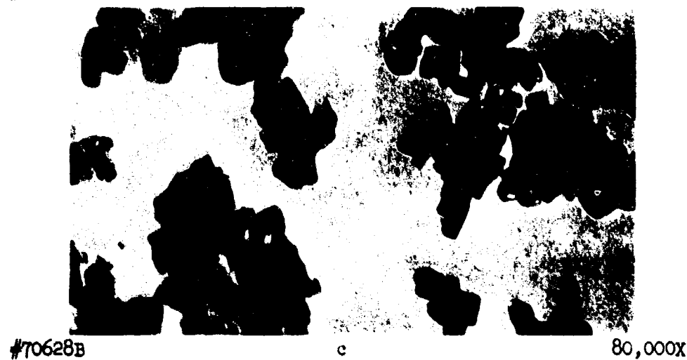
Figure 4. MgO Calcined from \text{Mg}(\text{OH})_2 in Rotary Vacuum Calciner at (a) 800^\circ\text{C} -1 hr., (b) 1000^\circ\text{C} -1 hr., and (c) 1200^\circ\text{C} -1 hr.
