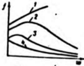
Figure 4.5. Friction coefficient f versus sliding velocity w for different specific loads [76]: 1) low specific load; 2,3) intermediate specific load; 4) high specific load.
