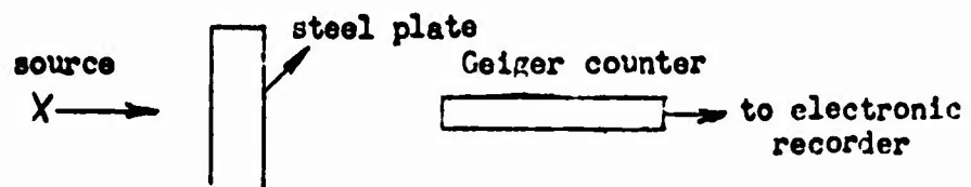
Fig. 4. Diagram of the principle of determination of thicknesses by Geiger method.
