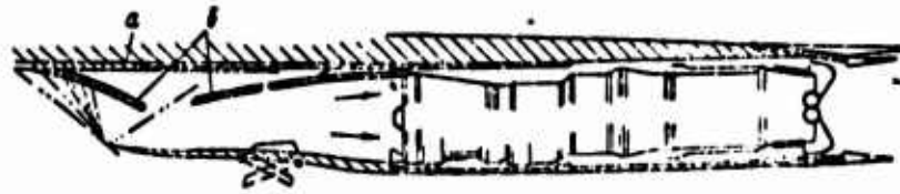
Fig. 5.24. Diagram of control of the intake of the TRD Bristol-Siddley "Olympus" 593 installed on the aircraft "Concorde": a) "takeoff" position; b) "supersonic flight" position.
