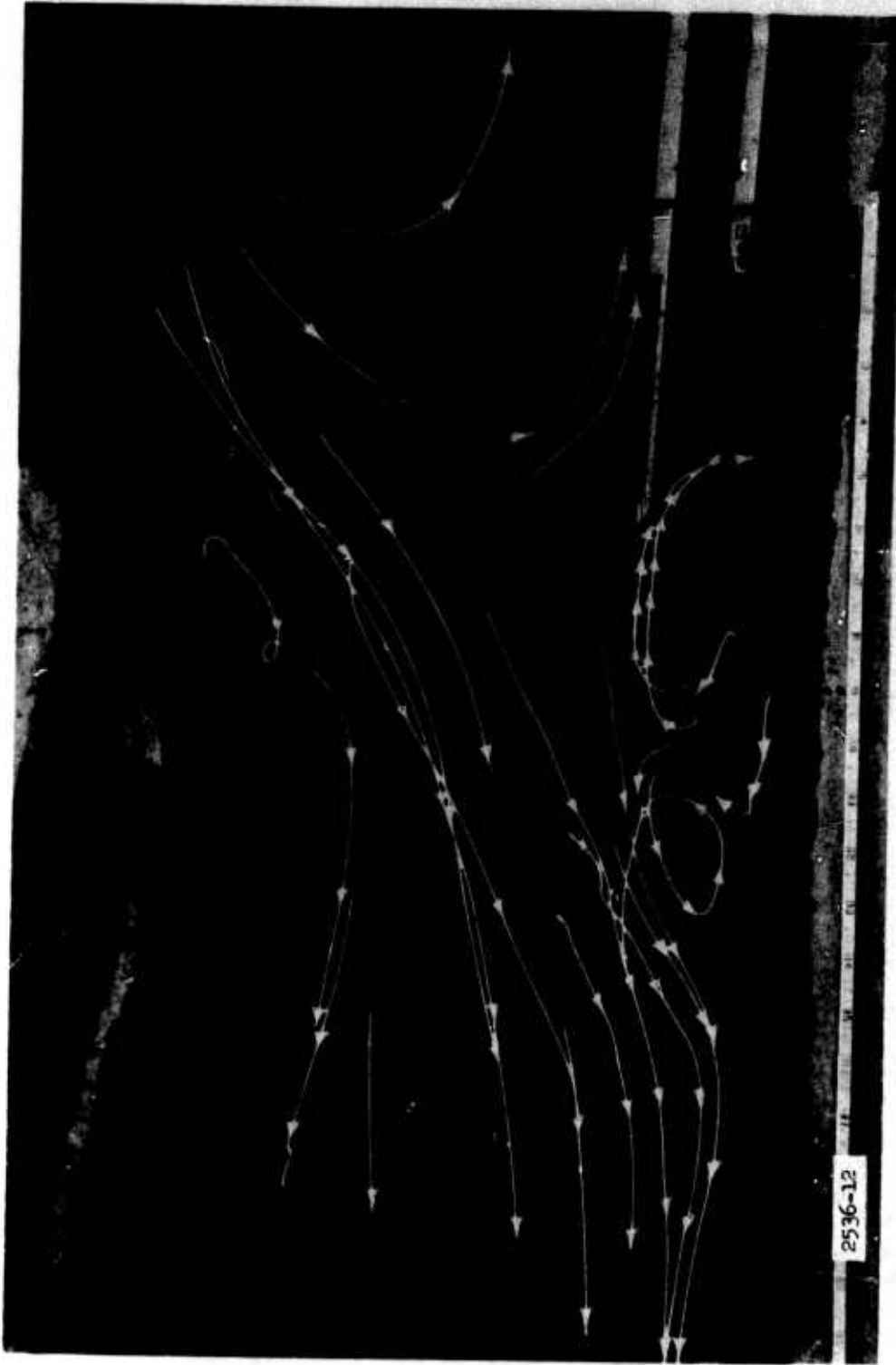
Photograph 2. Paths of floats (submerged 9 ft) during period 22-33 min after start of power release. Powerhouse discharge increased from 0 to 50,000 cfs in 6 sec (prototype). Numbers indicate average velocity in feet per second during 11-min period
