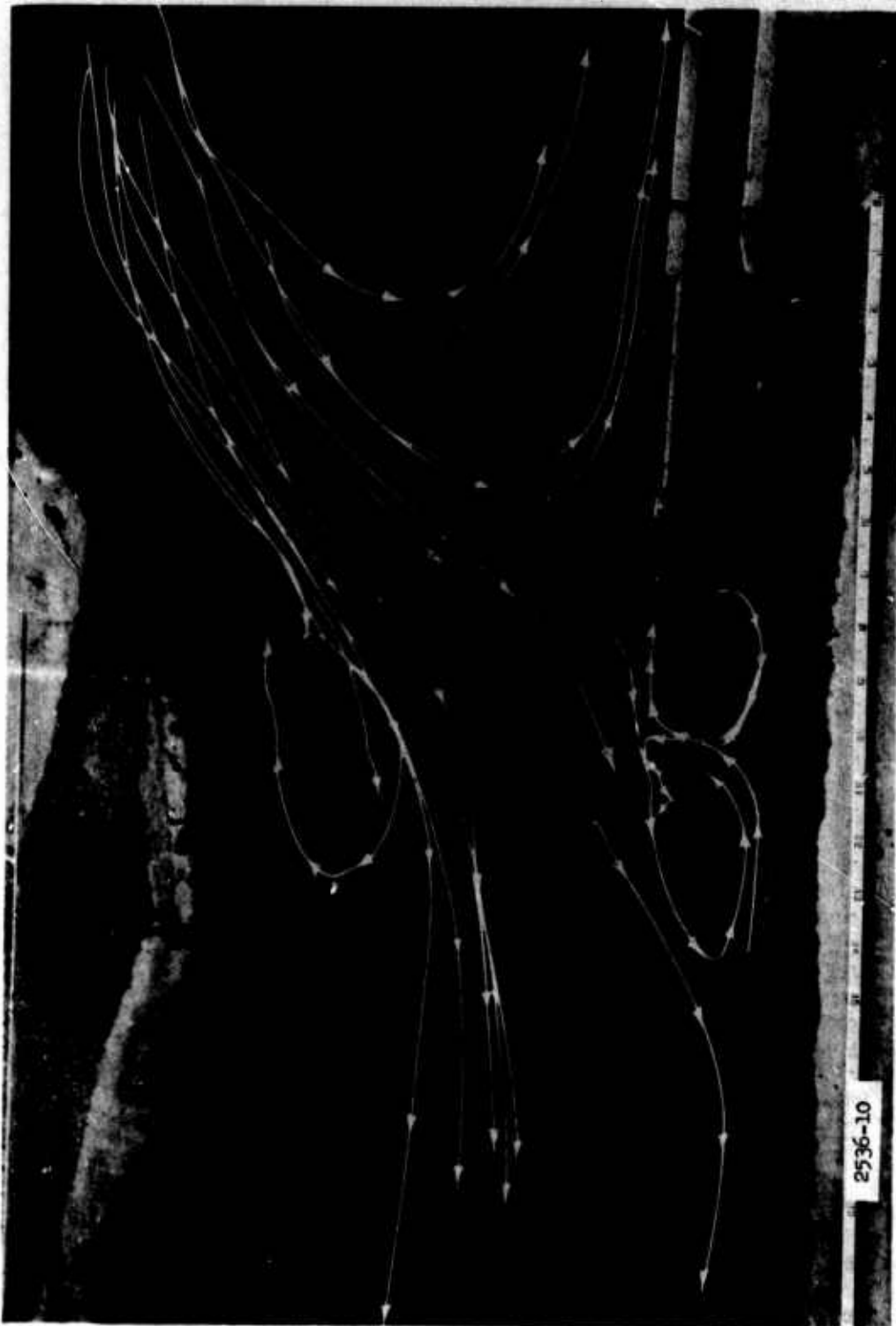
Photograph 6. Paths of floats (submerged 9 ft) during the period 44-55 min after start of powerhouse release. Powerhouse discharge increased from 0 to 50,000 cfs in 25 min (prototype). Numbers indicate average velocity in feet per second during 11-min period
