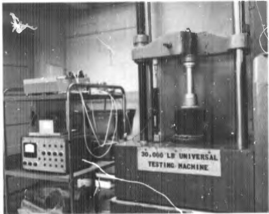
Figure 3.2 Slow-loading constrained compression test configuration.
