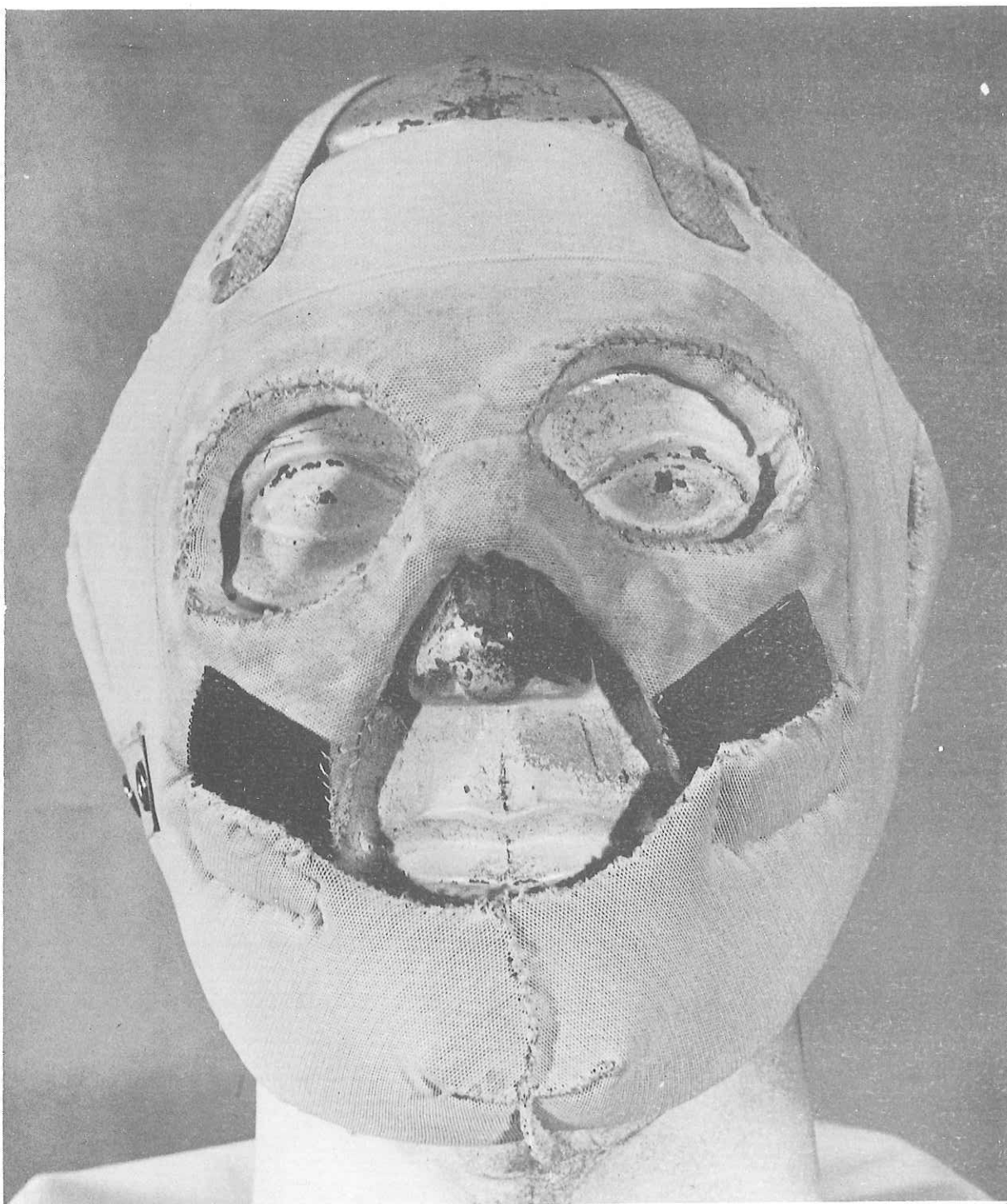
Figure 13. Facepiece Adjustment Approach Using Slits to Compensate for Face Length Variation
