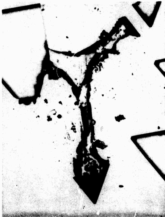
Figure II-9. This shows a triangular hillock that is attached by a Y-shaped web to the epitaxial layer of Growth No. 83, on a (III)-A substrate. The hillock was cleaved from the layer to expose the web. Infra-red micrography shows that all triangular hillocks on (III)-A substrates are similarly attached, but not the hexagonal hillocks of fig. 8 (b).
