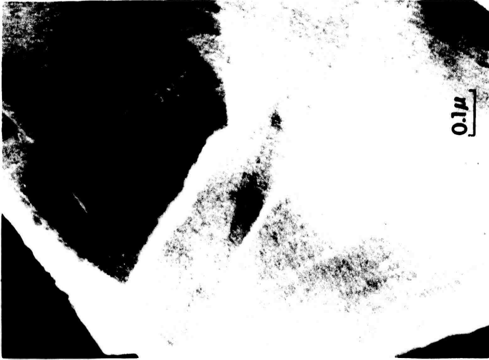
(d) A thin flake extracted from a cleavage surface (note that the flake is thin enough to be partially transparent to the beam thereby revealing some internal structure).
