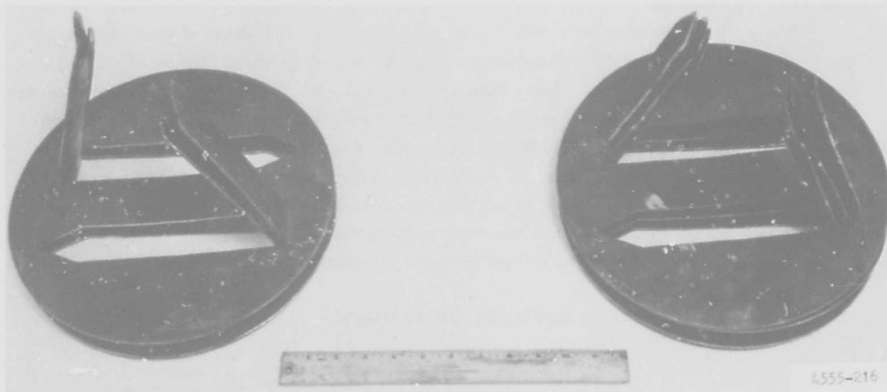
Fig. 8. Two-legged anchors stacked for packaging
