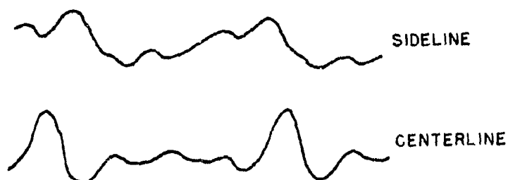
Figure 42. Measured Time History of Acoustic Pressure, Advancing Blade Side, 140 kt.
