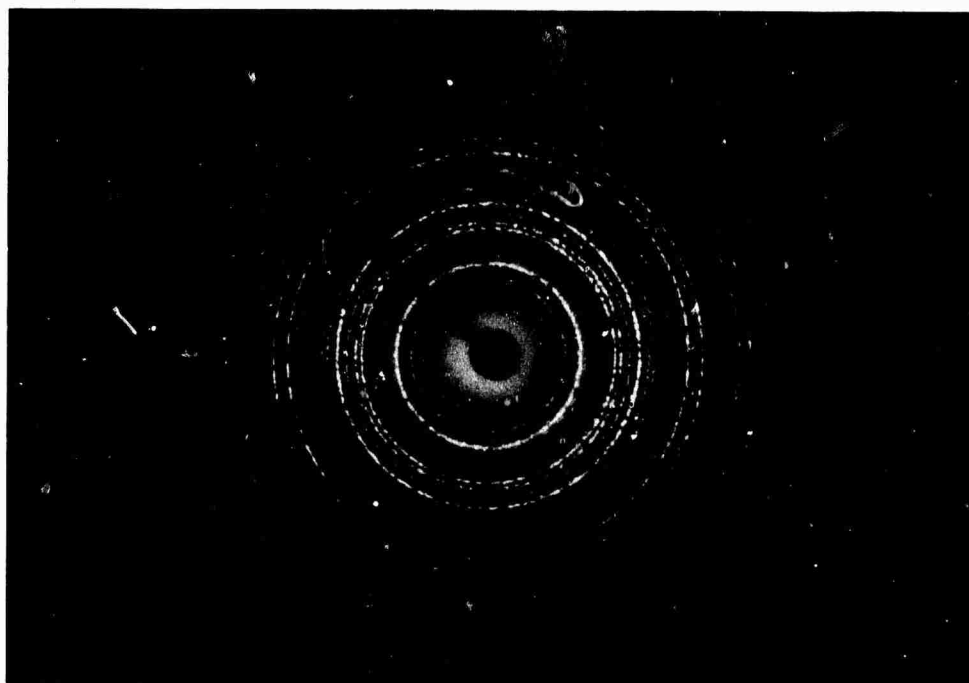
Figure 6.6 (b) SAD from Figure 6.3 (b) showing Te and GeTe
