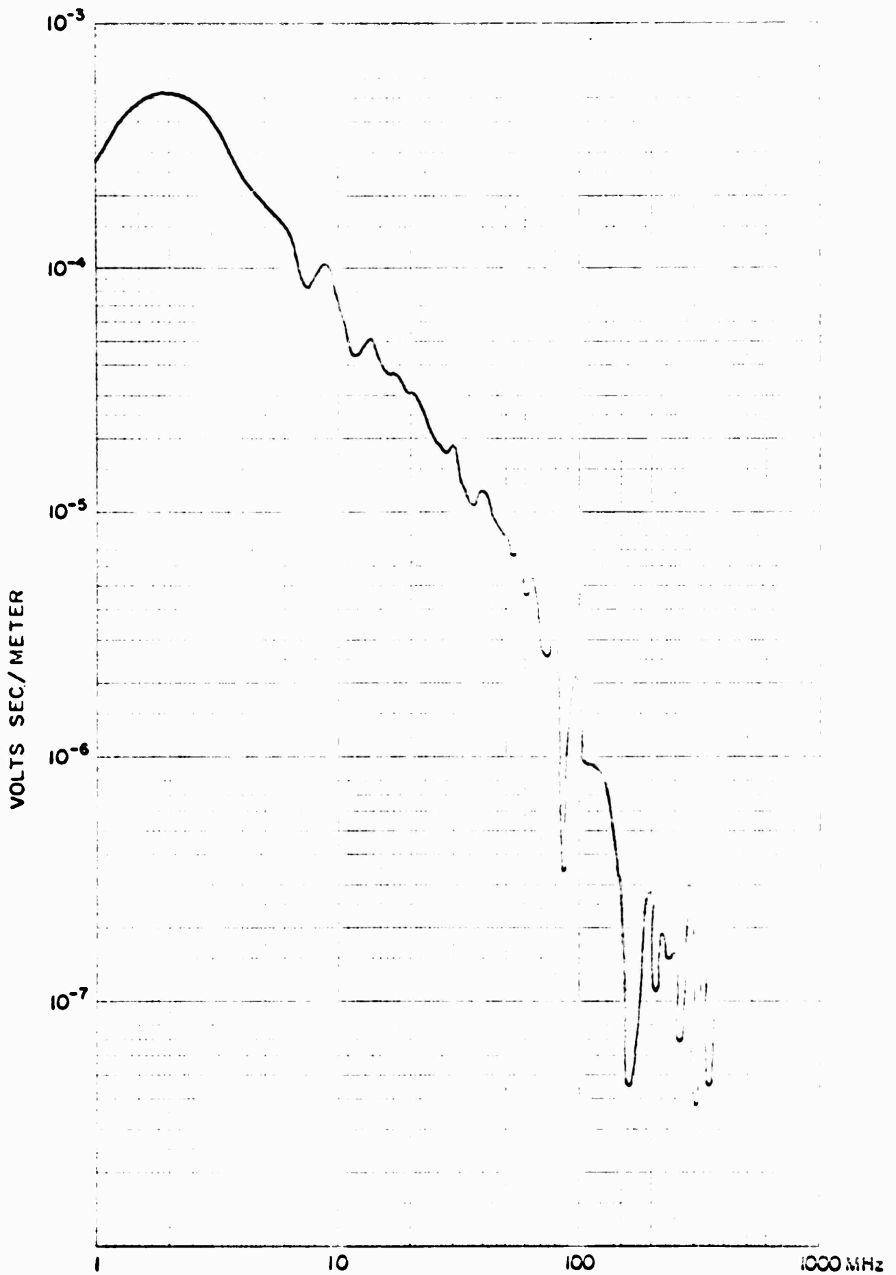
Figure 9. Spectrum of Pulse Transmitted with Large Vertical Antenna
