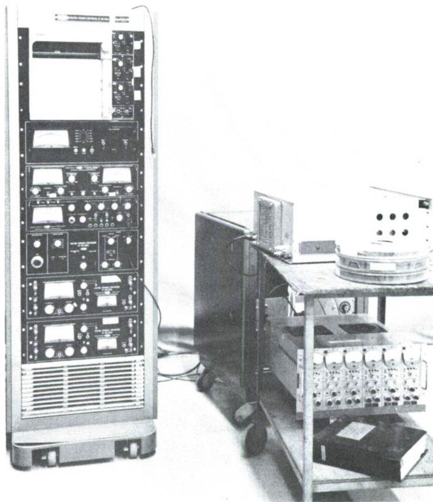
The SD1002B-33 Automatic Mechanical Impedance System and Charge Amplifiers
