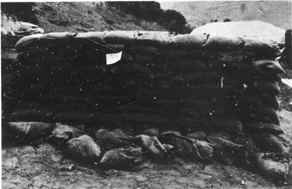
Figure F-11. Damage to sandbag wall from 81-mm mortar round at 10 feet.
