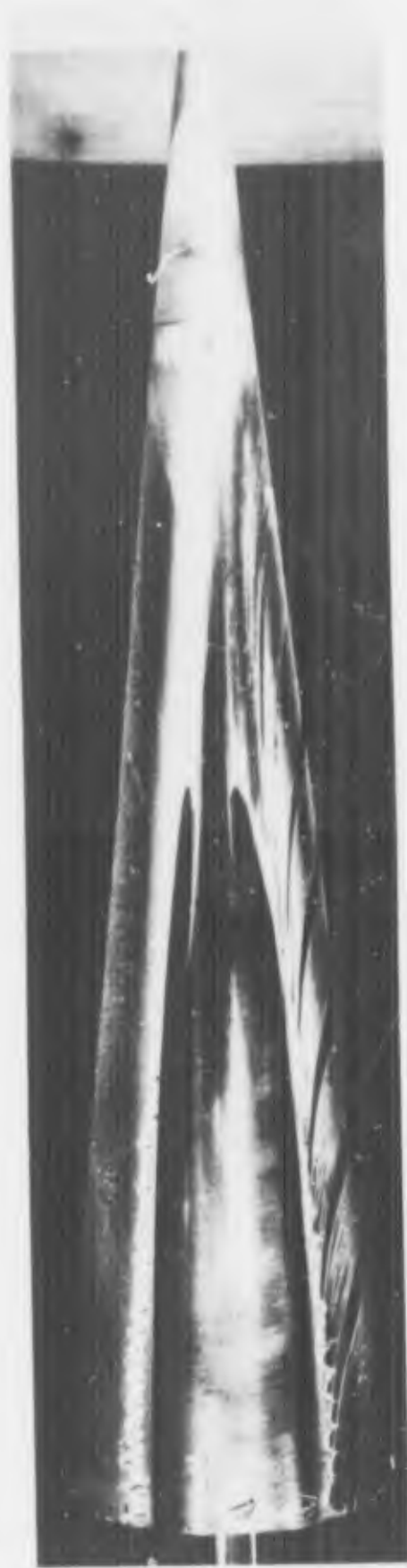
Figure 73. Oil Flow Photographs, Side and Leeward Views, 10% Bluntness, \alpha = 6 Degrees
