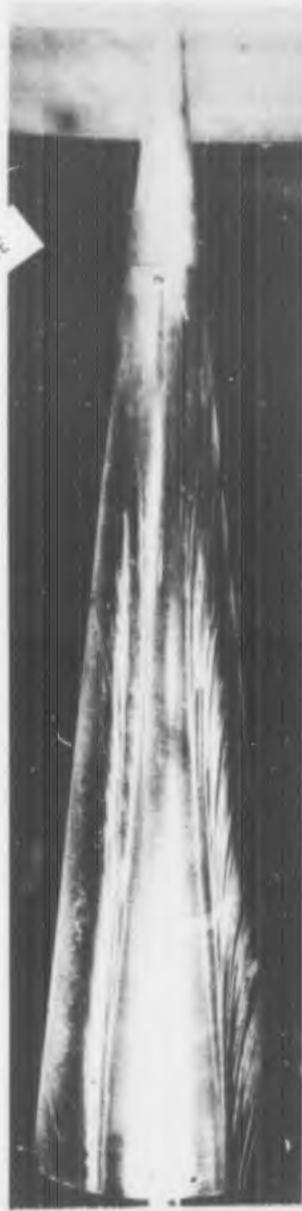
Figure 72. Oil Flow Photographs, Side and Leeward Views, 10% Bluntness, \alpha = 5 Degrees
