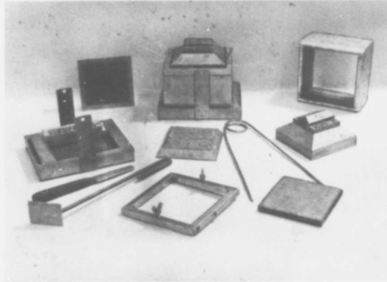
Fig. 23. Terzaghi's shear box
