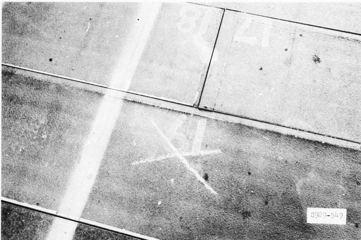
Photograph 13. Break in top skin of panel 19 adjacent to female connector after 450 coverages
