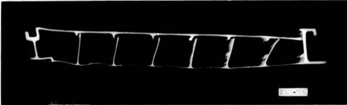
Photograph 21. Cross-section view of internal rib failures in panel 43 after 450 coverages
