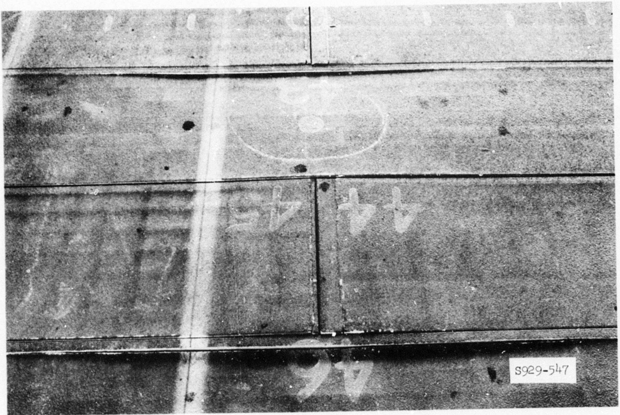
Photograph 11. Splits in top skin of mat after 450 coverages
