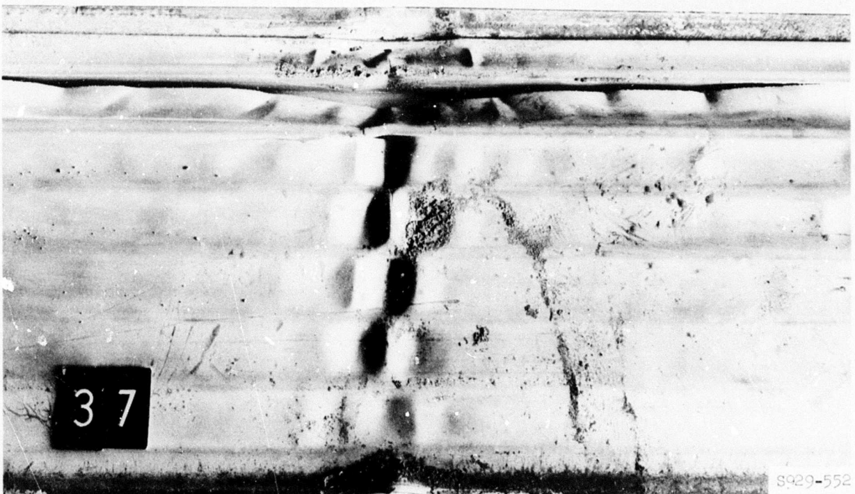
Photograph 18. Failures in bottom skin of panel 37 after 450 coverages
