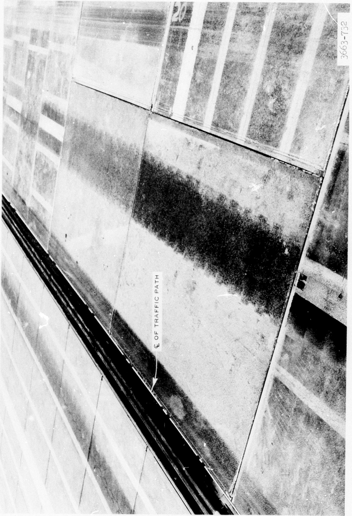
Photograph 8. Kaiser 4- by 4-ft aluminum honeycomb mat and Harvey modified AM2 in item 4, lane 1, after 100 passes
