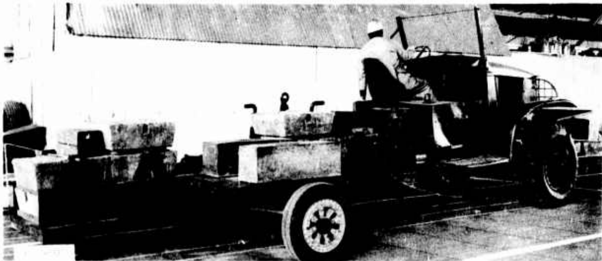
Fig. 6. Test cart with 27,000-lb single-wheel load with tire inflated to 400 psi
